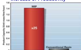
Figure 6. The diagram shows a 25 times higher product capacity in unit mass/liter per hour using a MIP packed column compared with a conventional resin. (Figure based on calculations performed by the customer)
